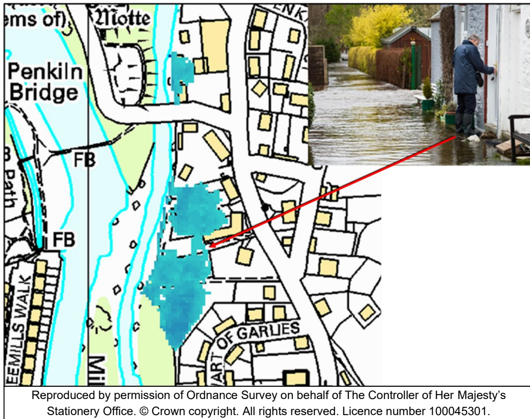
Figure 5: Known flood extents compared against modelled water levels
