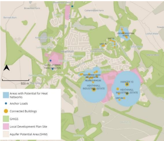
Figure 12-12: Potential Heat Network Zone, Dumfries Industrial Area
