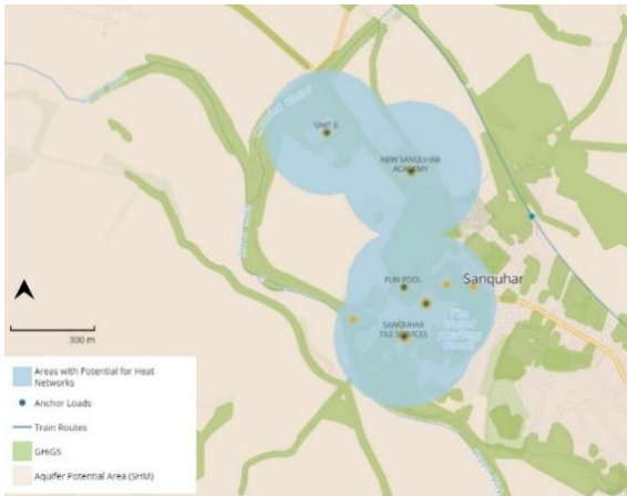
Figure 12-8: Potential Heat Network Zone, Sanquhar
